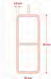
Front view of comparative extruded aluminum design
