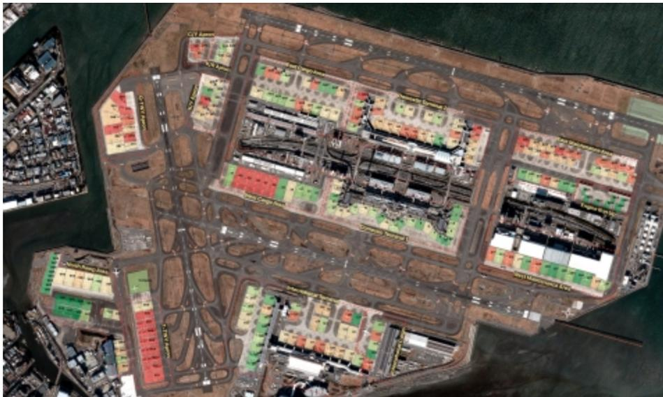
Using high-revisit satellite imagery, BlackSky’s Spectra AI has detected the utilization of major facilities at Tokyo’s Haneda Airport. Parking spaces shown in green are rarely used, while red indicates frequent occupancy. BlackSky customers can also understand inflow/outflow of cargo and monitor airline maintenance activity. (Photo: Business Wire)
