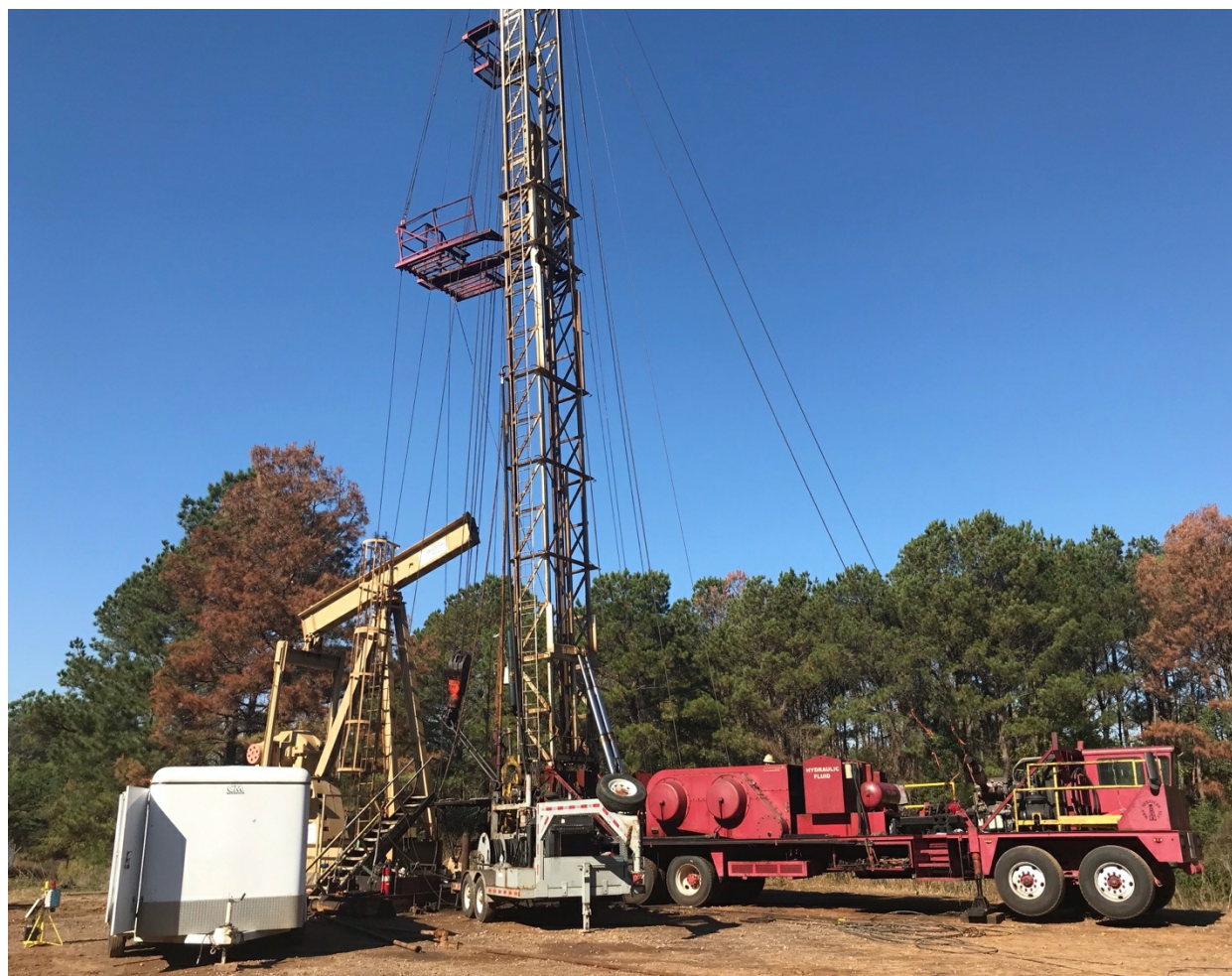
Figure 2: Workover rig at the pre-existing production well in East Texas. This rig was used to re-perforate the existing production casing to allow brine sampling from various zones in the Smackover Formation.
