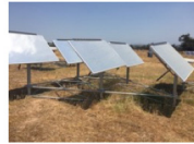
1) Off-the-Shelf Sun-tracking Heliostats (~4 acres per 400 kW)
