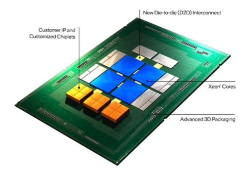
With the advent of advanced 3D packaging technologies, chip architects are increasingly adopting a modular approach to design – moving from system-on-chip to system-on-package architectures. This provides a way to partition complex semiconductors into modular blocks called "chiplets." (Credit: Intel Corporation)
