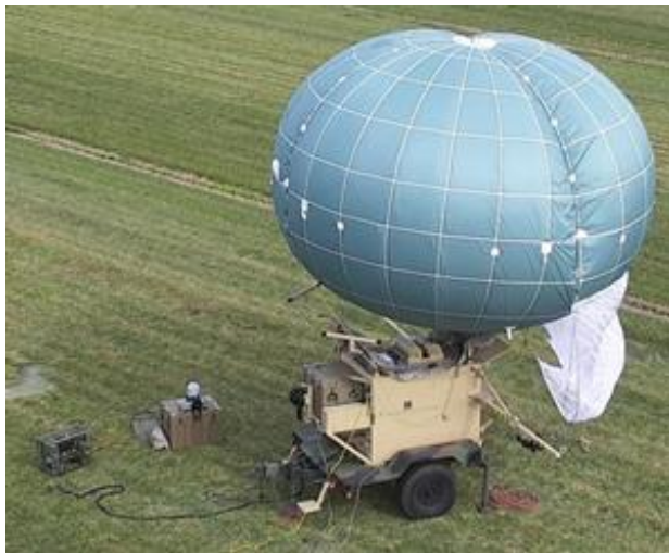
The Winch Aerostat Small Platform ("WASP") tactical aerostat from Drone Aviation Corp.
