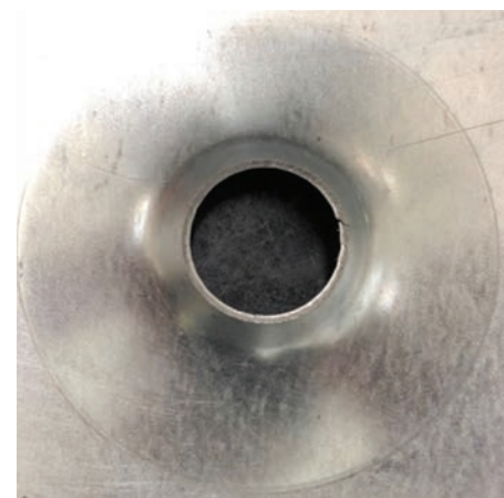
780CP Hole expansion test
