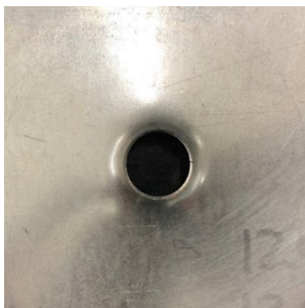
780DP Hole expansion test
