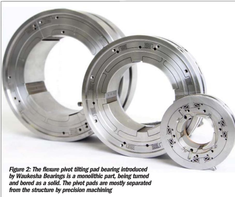
**Figure 2: The flexure pivot tilting pad bearing introduced by Waukesha Bearings is a monolithic part, being turned and bored as a solid. The pivot pads are mostly separated from the structure by precision machining**
