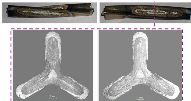
Fig. 6. Cross section of a 3-lobed Lightbridge rodlet after ~24 hours under dryout conditions during irradiation showing minimal damage in the valleys between the lobes.
