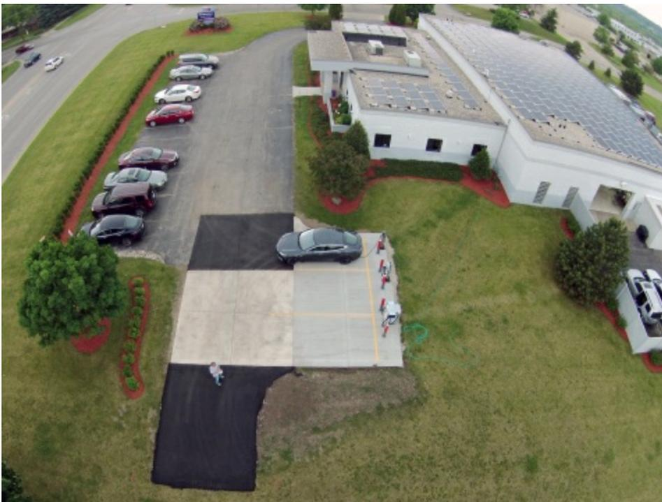
Solar panels help power more than 50 percent of Marshall Auto Body's annual electricity needs and comprise 10,000 square feet of its roof. (Photo: Axalta)
