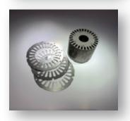
Cleveland-Cliffs' **Cold-Rolled Motor Lamination Steel** (CRMLS) products are Semi-Processed non-oriented electrical steels (NOES) designed for use in both small and large motors, generators, transformers, and electrical equipment. Standard grades available are Types 2 – 5 and are available in thicknesses of 0.018" –0.060" nom (0.46 – 1.52 mm)
