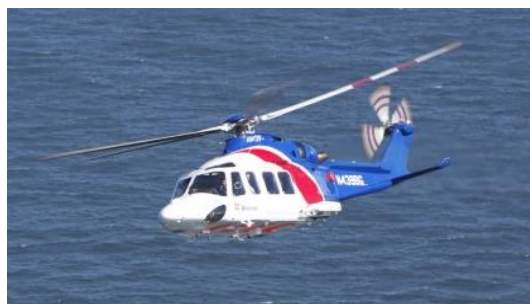
Medium Twin Engine: 12 passengers, 450 mile range, 145 knots
