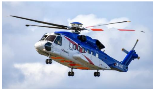
Heavy Twin Engine: 16-19 passengers, 500 mile range, 145 knots
