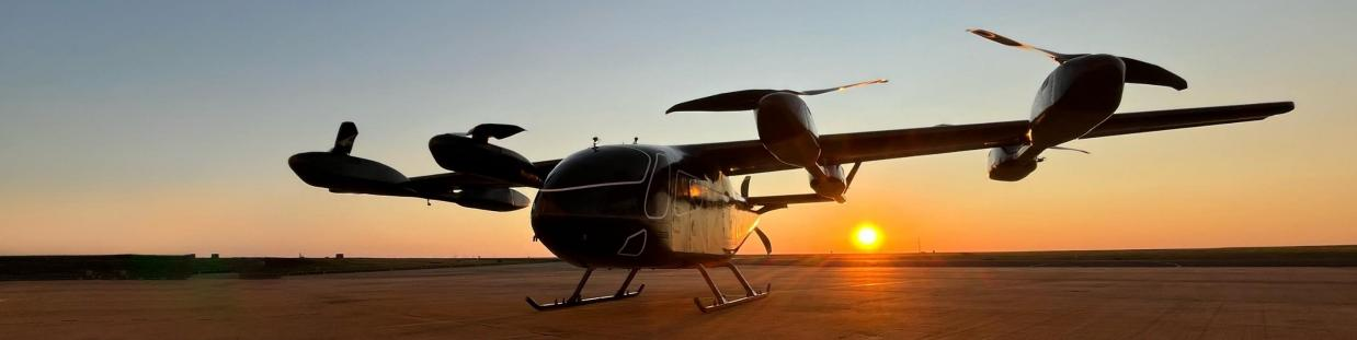
8 counter-rotating lifters (for controllability and high safely levels)
