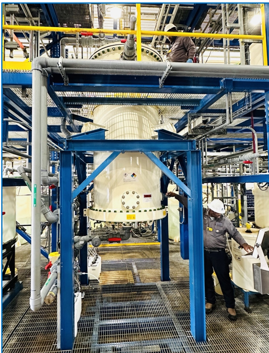
Figure 1 – Side elevation of operators working on the commercial-scale DLE column at Standard Lithium's Demonstration Plant near El Dorado, Arkansas.
