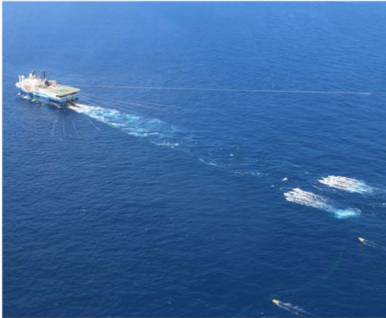
3D Seismic acquisition offshore Guyana
