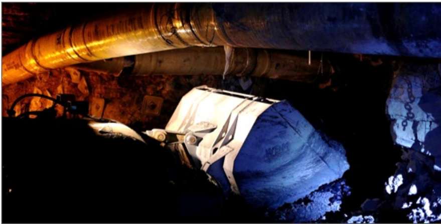
Image 2: Paringa loader mucking RoM material from the mine face
