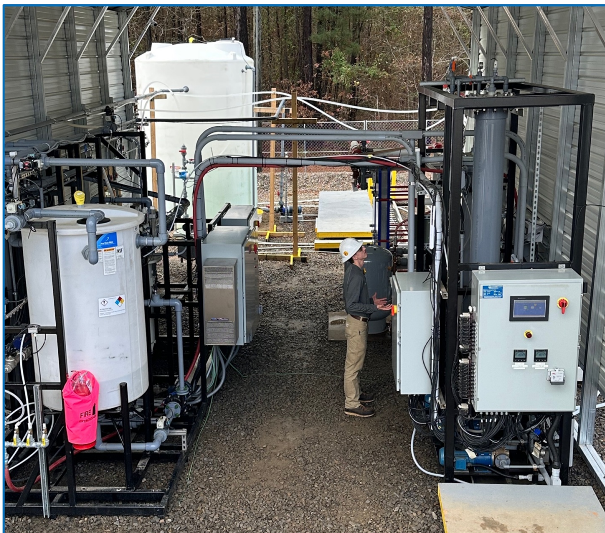
Figure 2 – Close-up of the brine conditioning and DLE steps at the field-based pilot plant.
