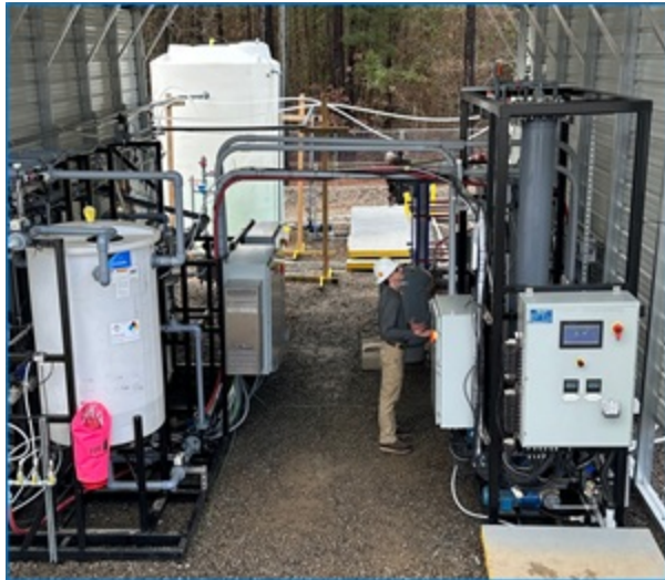
Close-up of the brine conditioning and DLE steps at the field-based pilot plant.
