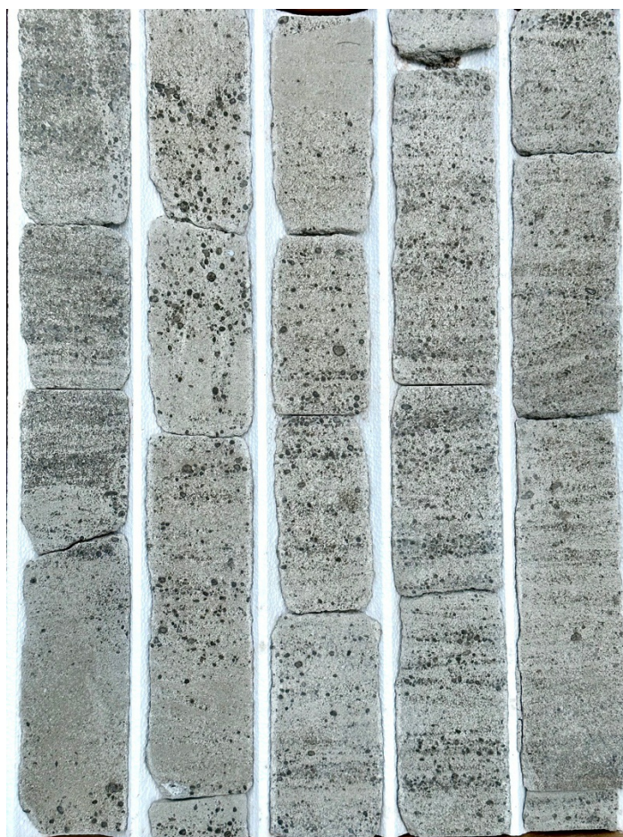
Figure 2: Examples of high porosity oolitic limestones from the Smackover Formation recovered from the Montague Well. This well is part of Standard Lithium’s current drilling program in the South West Arkansas Project.
