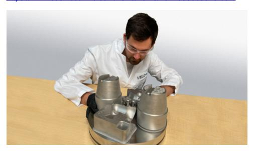
Engineer evaluating an M300 tool steel print of conformal cooled tooling and high pressure die casting inserts. These types of inserts are widely used to manufacture parts for the automotive industry. (Photo: Business Wire)
