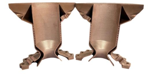
A cross-sectioned thrust chamber printed on a Velo3D Sapphire system in GRCop-42. The chamber walls contain internal channels for regenerative cooling. (Photo: Business Wire)
