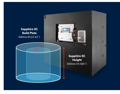
Sapphire XC, the new "Extra Capacity" large-format printer from VELO3D, will increase production throughput by 5X and reduce cost-per-part by up to 75%
