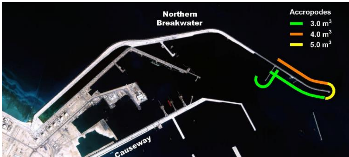
FIGURE 2: SECTIONS COVERED WITH ACCROPODES
