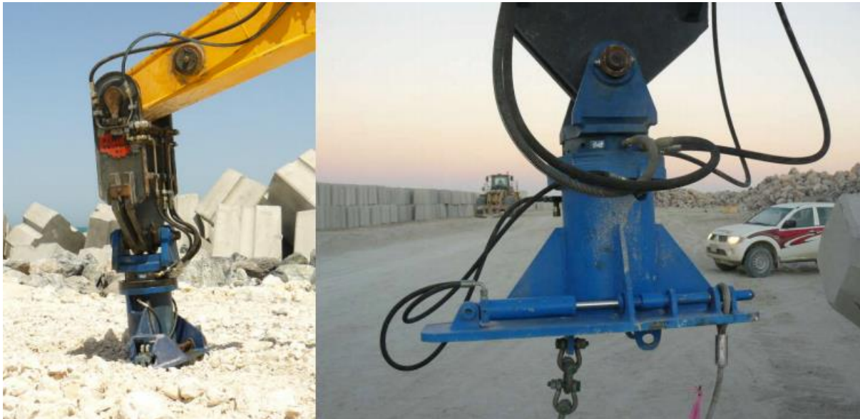
FIGURE 5: ROTATOR SYSTEM WITH DETAIL OF RELEASING SYSTEM (RIGHT)
