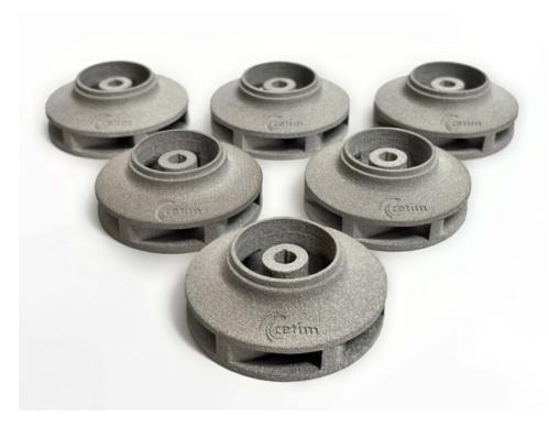
These complex water pump impellers, binder jet 3D printed in 304L on the Desktop Metal Shop System<sup>™</sup>, show the kind of complex geometries that can now be produced without tooling or machining. Desktop Metal, in partnership with CETIM, has now qualified 304L stainless steel for processing on the Shop System. (Photo: Business Wire)
