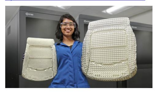
FreeFoam is currently being printed exclusively on the ETEC Xtreme 8K topdown DLP printing system, with broad commercial availability slated for 2023. ETEC is Desktop Metal's industrial polymer brand.
