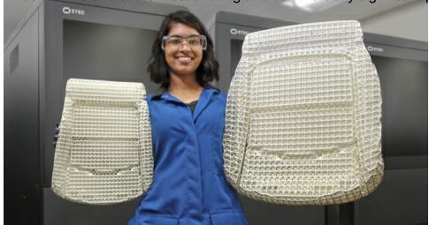
These automotive seats were 3D printed in an innovative new FreeFoam<sup>™</sup> photopolymer resin that can be expanded in an oven after printing. The seat on the left showcases the material after 3D printing but before expansion, while the seat on the right shows the fully expanded seat after a quick trip through an oven. The seats were 3D printed on the ETEC Xtreme 8K topdown DLP printer shown in the background. (Photo: Business Wire)
