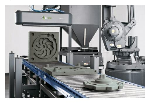
ExOne, which was acquired by Desktop Metal in late 2021, is the leading digital sand printing solution provider for foundries. The new S-Max Flex combines ExOne's sand printing expertise in process and materials with proprietary Desktop Metal SPJ technology in an affordable architecture to deliver new value to foundries that have long wanted an S-
