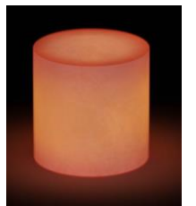
Printed TRISO nuclear fuel for Gen 4 MMR/SMR
