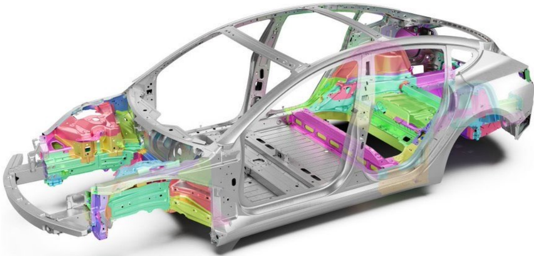
Model 3 body structure 171 pieces of metal highlighted
