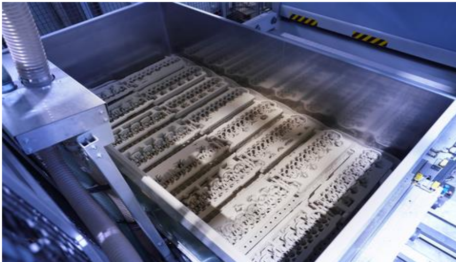
BMW Landshut plant hosts one of the largest super fleets of DM's ExOne Exerial printers for mass production of metal parts. These complex parts have geometry that can only be made with 3D printing and are used in nearly every vehicle produced by BMW
