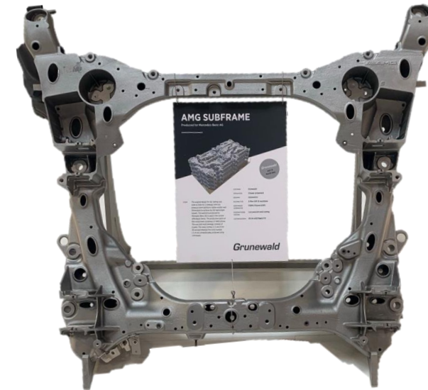
Mercedes Benz AMG subframe manufactured by a DM customer who employs a super fleet of 11 S-Max printers. This single 3D printed digital casting reduces weight by consolidating multiple previously stamped and welded sheet metal parts into a single part
