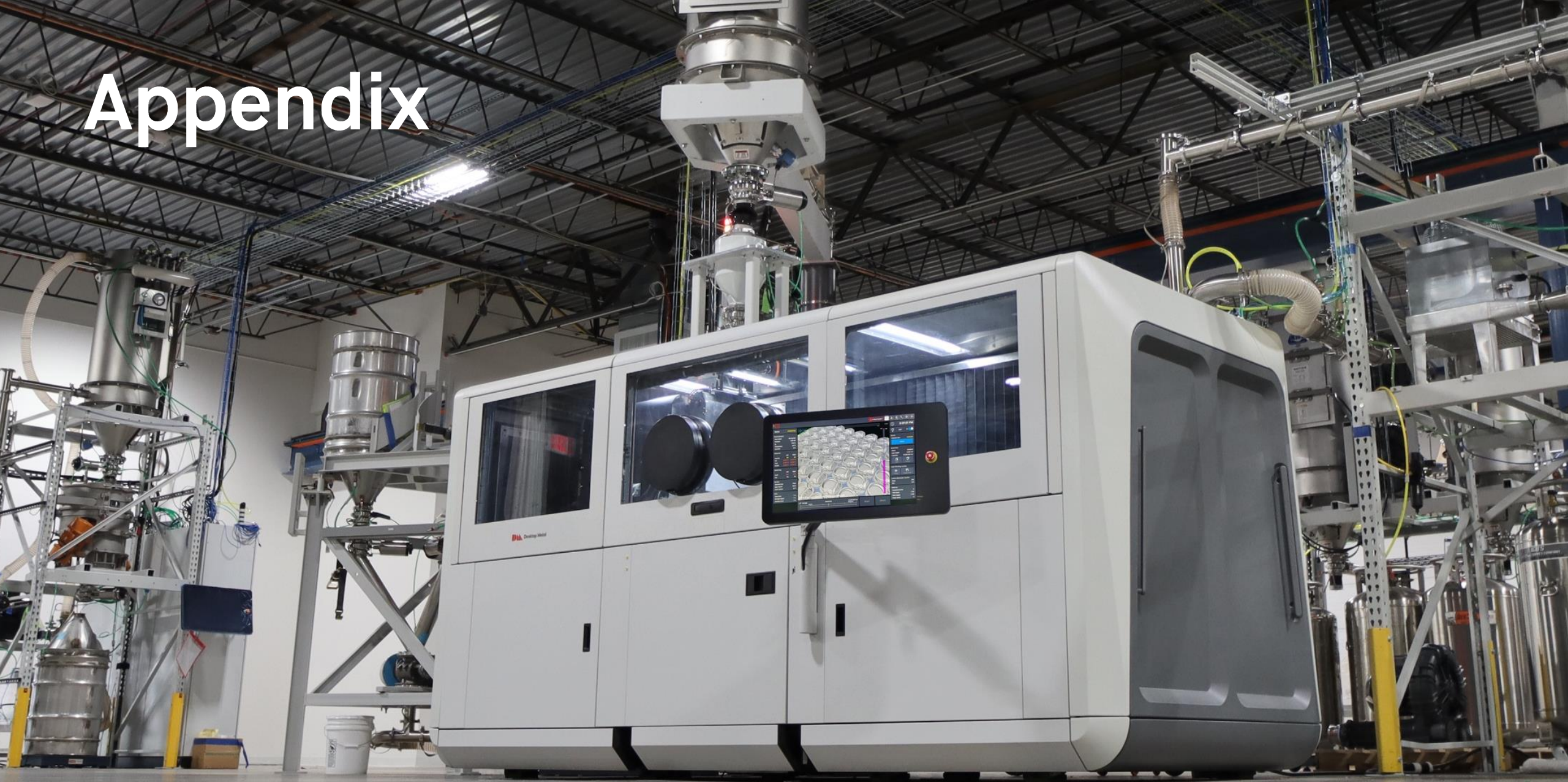
Desktop Metal Production System P-50 printer and auxiliary equipment
