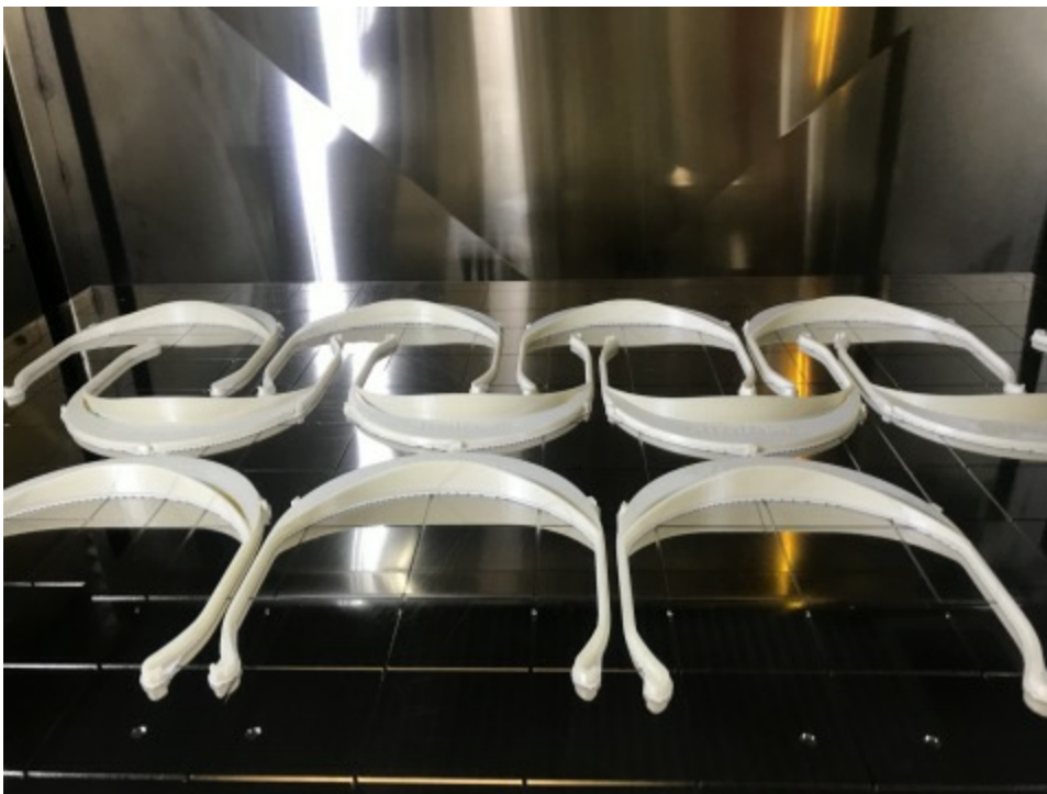
A tray of face shield visors being 3D printed by Stratasys. Thousands are now being produced by Stratasys or its coalition partners. (Photo: Business Wire)
