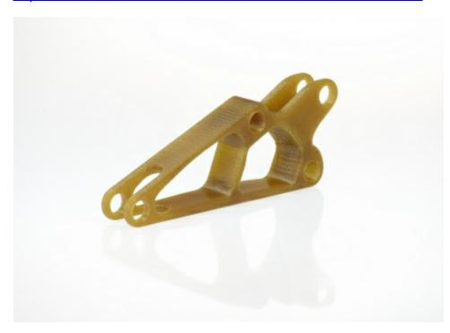
Antero 800NA (PEKK) bracket, used to mount hydraulic components in an aircraft wing. It replaced a machined PEEK part, eliminating the material waste of the subtractive process. (Photo: Business Wire)
