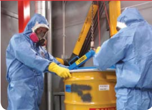
Drum receipt inspection station
