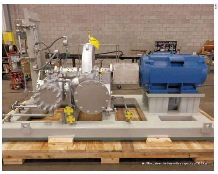
speeds and pressures. But, steam turbines at 15 to 35,000 horsepower can go five to seven years before they need any internal cleaning."
