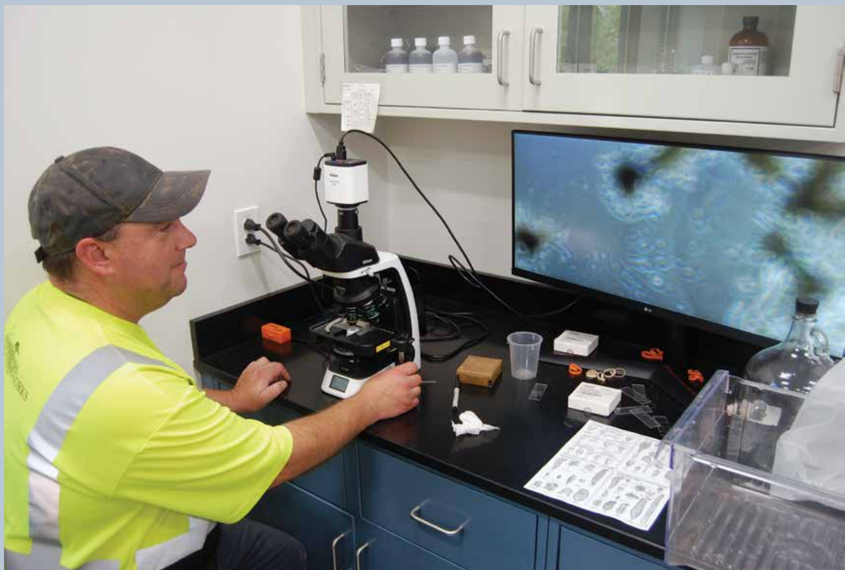
Microscopy is essential to process monitoring at the Wausau Wastewater Treatment Facility. Jason Schill, lab technician, views microorganisms on a large-screen display.
