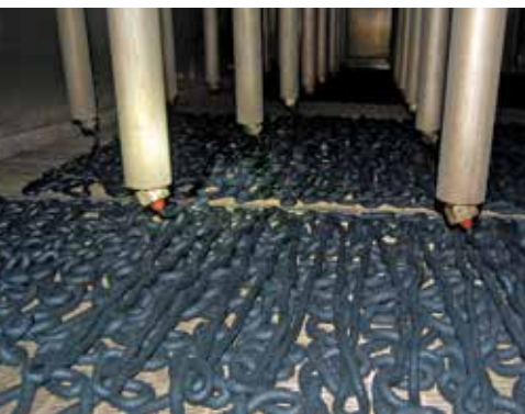
Biosolids are processed in a BioCon thermal drying system (Veolia Water Technologies). The inset photo shows biosolids being dried by indirect convective heating.
