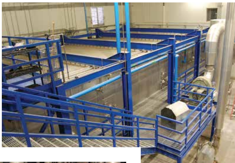
Biosolids are processed in a BioCon thermal drying system (Veolia Water Technologies). The inset photo shows biosolids being dried by indirect convective heating.
