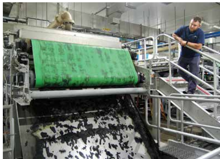
Austin Trinko, operations technician, with one of the facility's two belt filter presses (Charter Machine Co.) that dewater biosolids to 18-22% before transfer to the thermal dryer.
