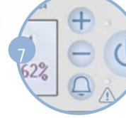
Set the flow setting to the flow rate prescribed by your clinical professional. The flow setting can be changed by pressing the circular flow setting buttons that are marked with "+" and "-" symbols. Position the nasal cannula on your face and breathe normally through your nose.
