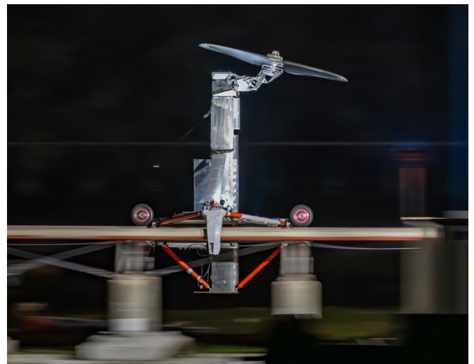
Our 'Whirly' propulsion system test asset, used to conduct endurance testing.
