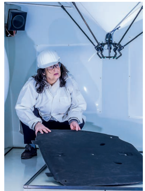
“Tests show that our original, non-bio-based VEF systems can outclass standard high resilient (HR) foams at lower frequencies.”
