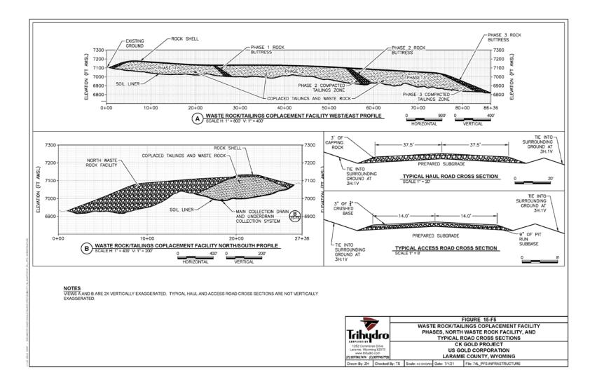
**Figure 15-5 Facility Cross Sections**
