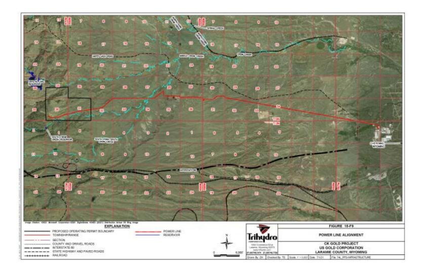
**Figure 15-9 Proposed Powerline Alignment**
