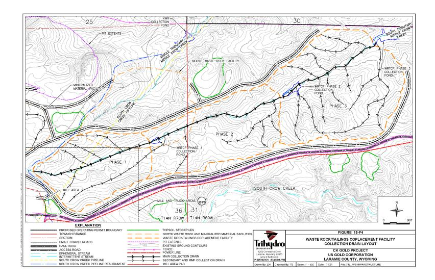
Figure 15-4 WRTCF Collection Drain Layout
