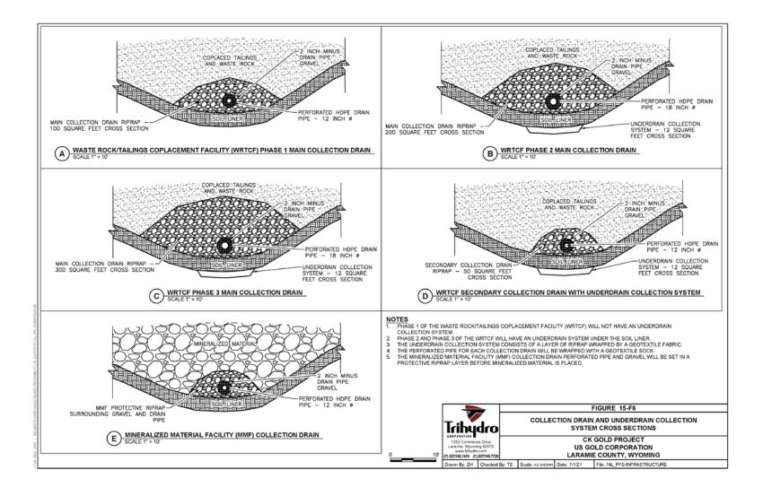
Figure 15-6 Drain System Cross Section
