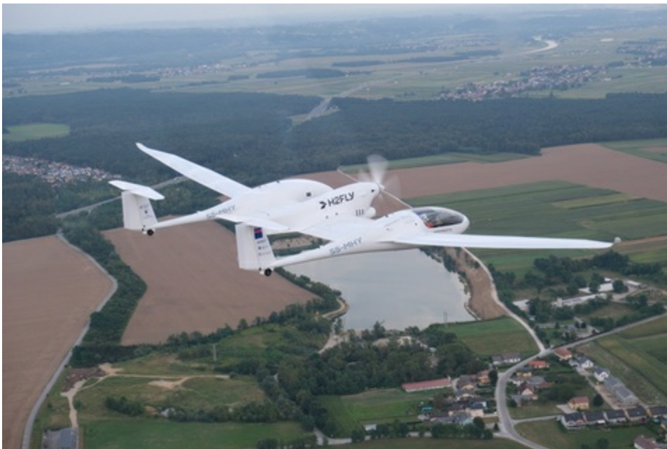
H2FLY's HY4 electric demonstrator aircraft flying above Maribor, Slovenia, powered by liquid hydrogen. Courtesy of H2FLY
