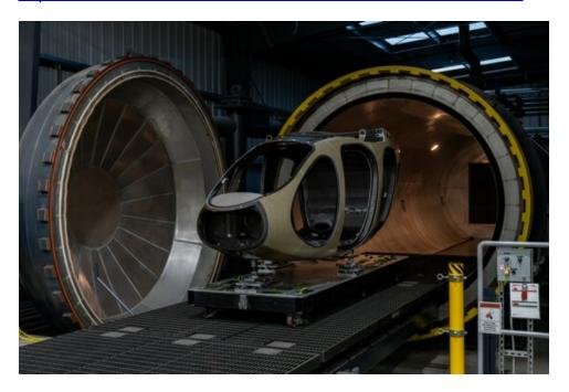
The fuselage of the first aircraft to be produced on Joby's pilot manufacturing line in Marina, CA, heads into a large autoclave to be post cured at a precise temperature and pressure. Credit: Joby Aviation.
