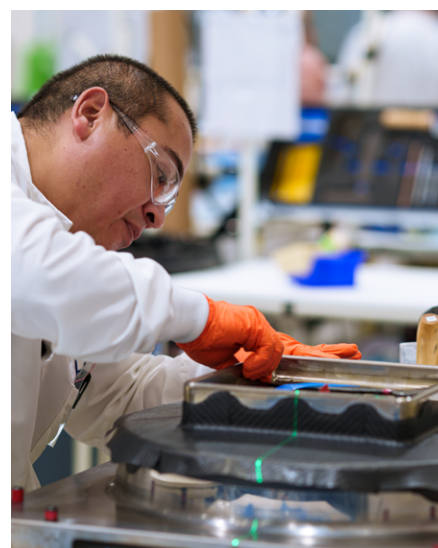
A Joby team member uses laser guides to precisely lay up a carbon fiber ring frame.
