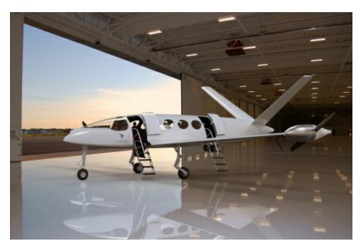
Eviation electric aircraft designed to take 9 passengers up to 1,000km at more than 240kts - all at the price of a train ticket (Photo: Eviation).
