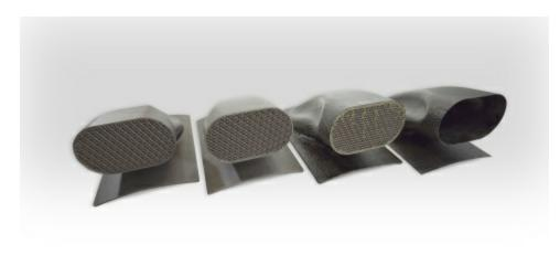
Sacrificial tool used to create a hollow inlet duct by Swift Engineering using Stratasys' new ST-130 material (Photo: Business Wire)
