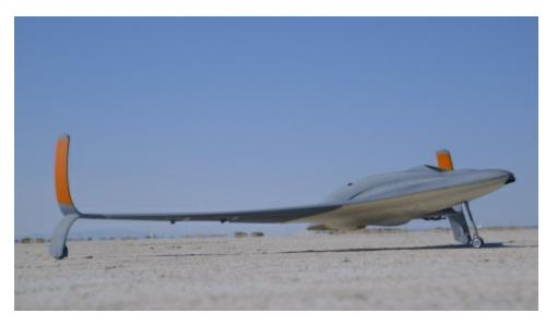
Making its global debut at the Dubai Airshow, Aurora Flight Sciences' highspeed UAV is 80% 3D printed with Stratasys additive manufacturing solutions. Photo: Stratasys
