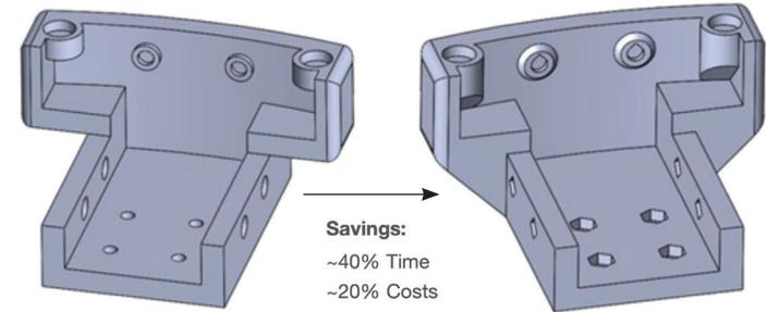
Adding self-supporting angles where possible makes soluble support redundant, since the model material is “self-supporting,” a key feature of FDM technology. As shown here, relatively minor changes can vastly cut costs and printing times.
