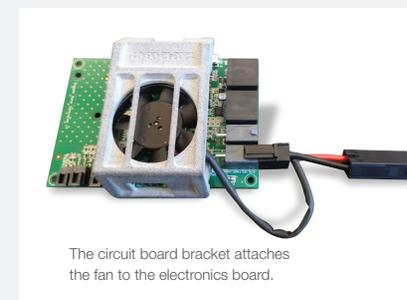
The circuit board bracket attaches the fan to the electronics board.
