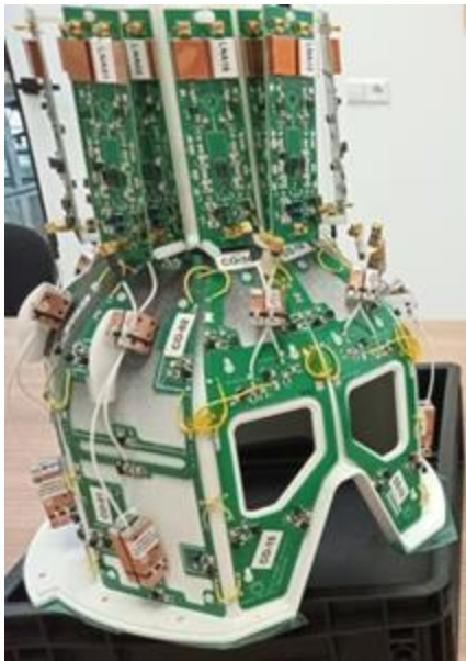
Tesla Head Coil (Tesla Dynamic Coils BV) Photo Courtesy of Alzamend Neuro, Inc. All rights reserved and proprietary, @2025
