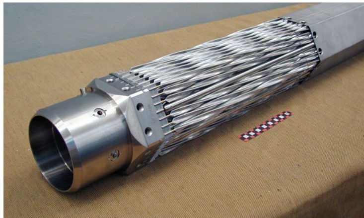
Fig. 3. Photo of the 108-rod seed-assembly consisting of 3-lobed, metallic, helically twisted Lightbridge Fuel rods used for thermal-hydraulic and vibration testing.
