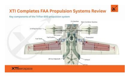
Engineering experts from XTI Aircraft Company, a subsidiary of XTI, and the FAA reviewed the TriFan 600 aircraft's propulsion system and compliance approach for the engines, drive train, fuel system, propellers, engine compartments and structural mounts for the drive train. The Tech Fam addressed key certification areas such as engine fire containment, bird strike impact, cabin occupant safety, fuel management, and instrumentation including sensors to detect system issues.
