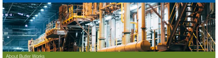
Butler Works is located in western Pennsylvania, a one-hour drive north of Pittsburgh. The facility produces stainless, electrical and carbon steels. Melting takes place in an electric arc furnace (EAF) that feeds an argon-oxygen decarburization unit for specialty steels. A ladle metallurgy furnace feeds two double-strand continuous casters. The buildings housing electrical-and stainless-steel melting and casting, hot-roll, cold-roll and finishing operations measure 3.5 million square feet.
